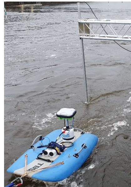
Testing with the UoE ADCP (front), and Kinetic Hydro flowmeter (behind) at Pinkston Watersports.
