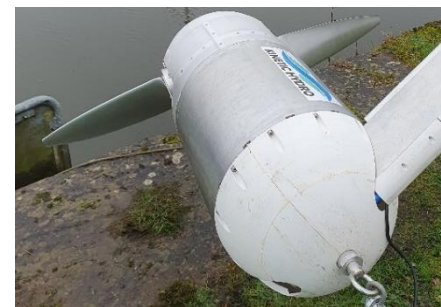
The Pitch Control Turbine on test in the workshop (top) and at Pinkston Watersports (below)
